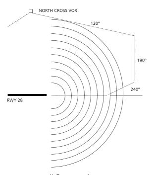
Figure 1 Radar vectors to an ILS approach
